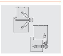
Application: 11R Ø 15-010-Adjustable hinge with security screws
