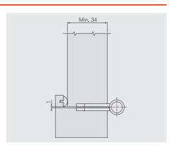
Application: 11R Ø 15-034–Adjustable hinge right hand for self closing system
