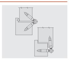
Application: 11R  $\emptyset$  20-017–Adjustable hinge with security screws
