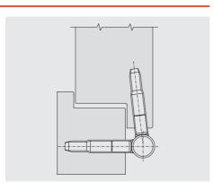
Application: ATC Ø 15-Self closing mechanism left and right hand
