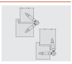
Application: 11R Ø 20-009-Adjustable hinge with security screws
