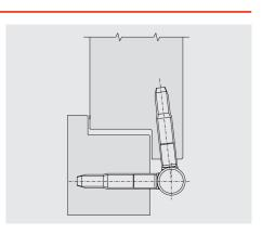
Application: 11R Ø 15-Adjustable hinge for self closing system
