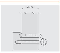
Application: 11R Ø 20-002-Adjustable hinge right hand with security screws
